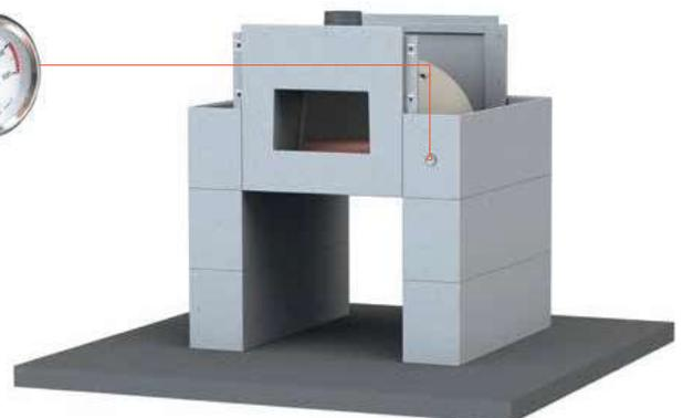
**7. Installation of side elements and the chamotte bottom.**
